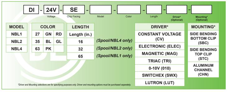
Example: DI-24V-SE-NBL2-35-16-CV-TBC = Diode LED, 24V NEON BLAZE<sup>m</sup> 2.44 w/ft. 3500 CCT, 16.4' long, 96" Lead Wire, and with a Constant Voltage Driver, and Top Bending Bottom Clips.
